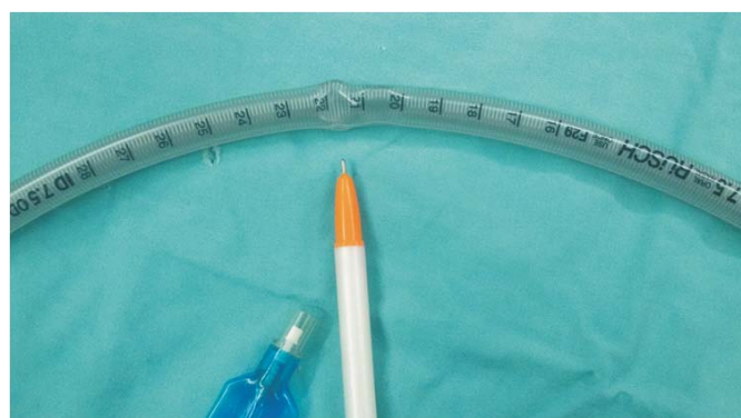
FIGURE 1 : 1. Armored tube in partial kinking when the tube is straight. (as shown in orange tip of pen between 21-22 markings)
